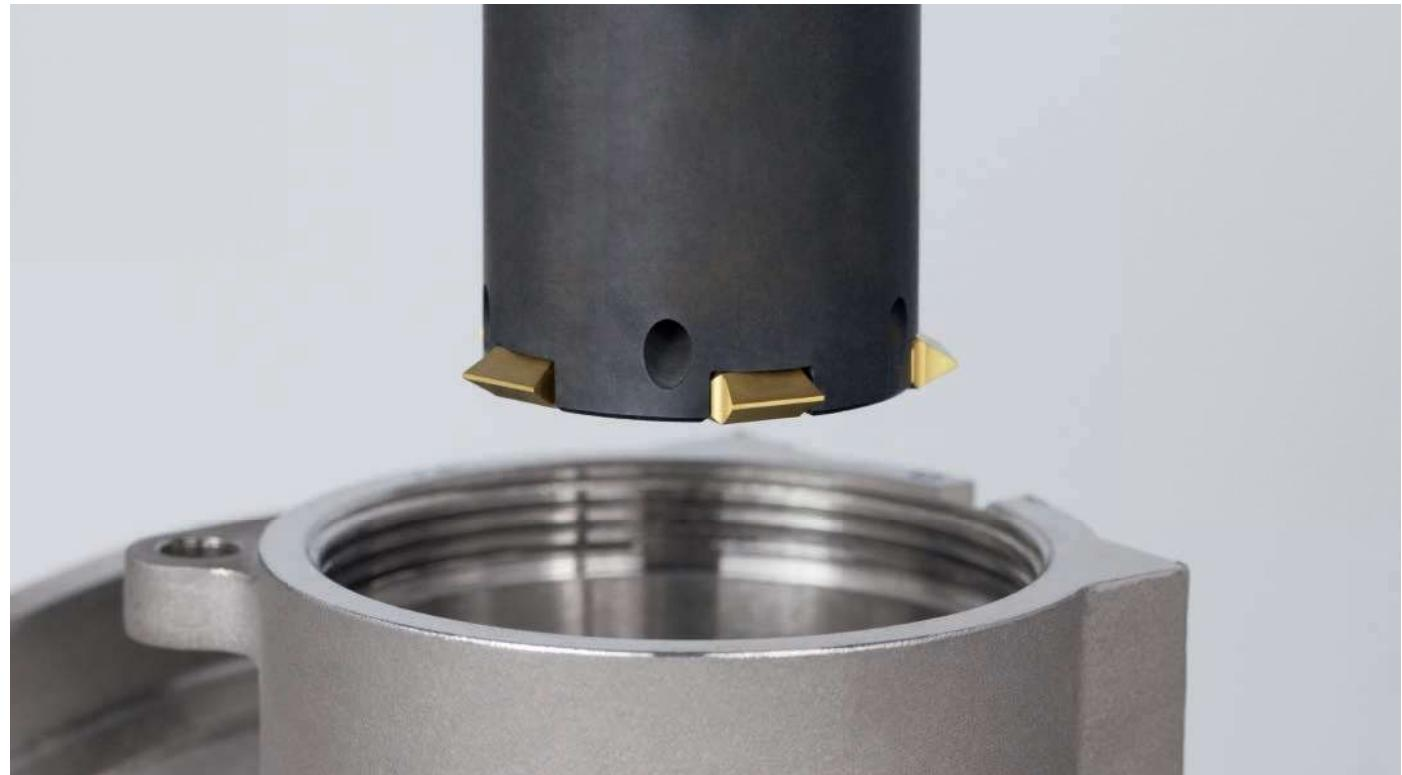
**Gewindefräsyklus · Thread milling cycle**
